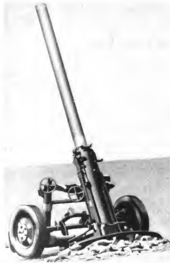
Figure 6-30. Heavy mortars. The 240-mm heavy mortar (below), with a range of 10,000 m, is large enough to fire nuclear or chemical shells. The 160-mm heavy mortar (above), towed on a wheeled carriage, has a maximum range of about 8,000 m.
